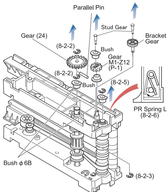
7) Pull out the Guide R PU upward, then remove Timing Belts.
