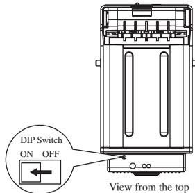
9. Set the READ/WRITE TOOL DIP switch setting Nos.5 and 6 ON and then supply the power to the READ/WRITE TOOL.
